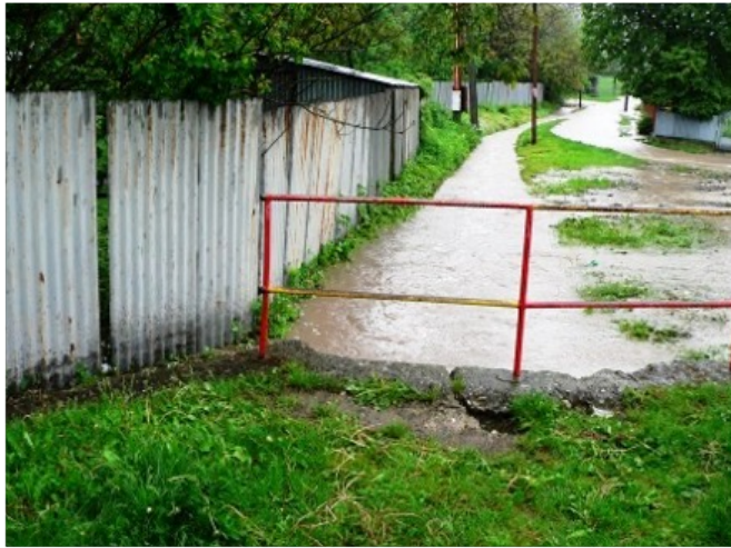
Left: An impermeable asphalted pavement and road allow the rainwaters to rush down faster, forming a flooded trail, stopped by a berm temporarily.
